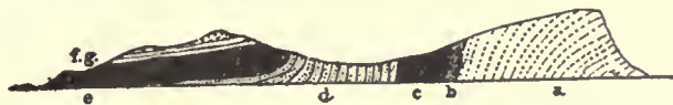
FIG. 1.—Section of the Isle of Wight—a Monoclinial Curve. a , Chalk; b , Woolwich and Reading beds; c , London clay; d , Bagshot series; e , Headon series; f , g , Osborne and Bembridge series.
